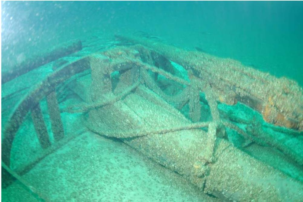
Figure 24. Foremast with top, trestle trees, cheeks, futtock band, truss, sling, and yard visible.
