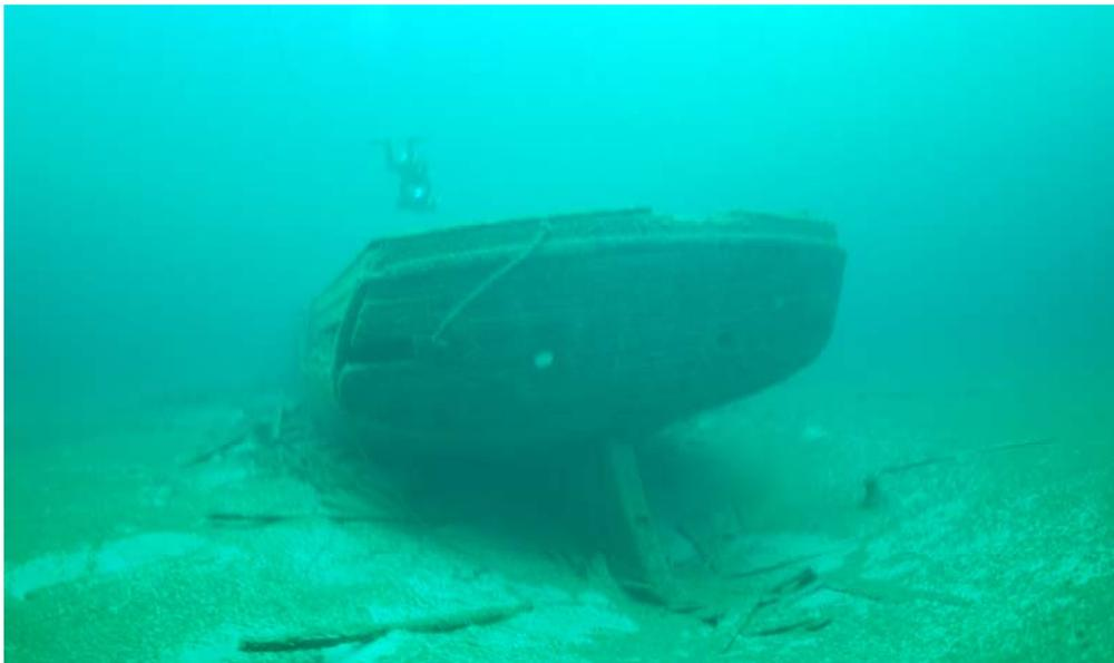
Figure 23. The transom is intact, but dislodged at the port quarter.
